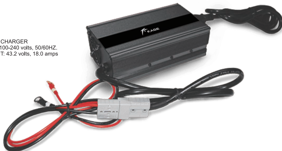
36V 18A CHARGER INPUT 100-240 volts, 50/60HZ. OUTPUT: 43.2 volts, 18.0 amps
